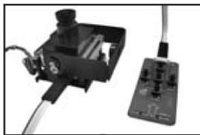
Connecting OSD Control Board to the Camera Module
