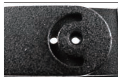
Replace the bracket onto extended arms by positioning on the adjusting holes desired.
