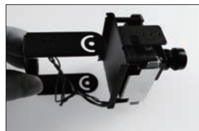
Remove the bracket out of the camera.
