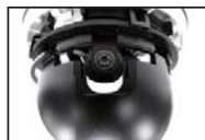
Install the Dome Liner on the Camera Module
